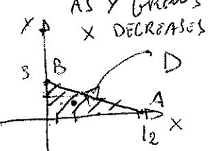
$$\text{Volume} = \iiint_{\text{Plane}} dV = \int_0^3 \int_{12-4y}^{12} 4 - \frac{1}{3}x - \frac{4}{3}y \, dx \, dy$$
